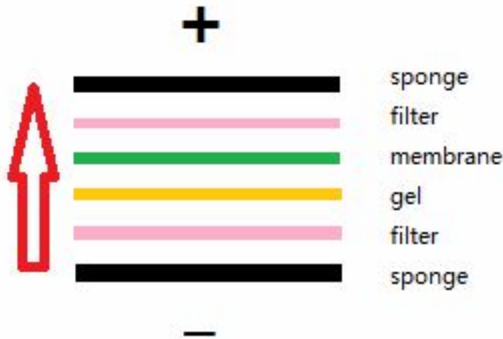
Figure 3: The “sandwich blot” for protein samples blotted electrophoretically to a PVDF membrane. “+” referred to the positive electrode, “-” represented the negative electrode. After building the electrophoretical field the proteins are moving from the “-” to the “+” field as the red arrow indicates, and were finally stopped by the PVDF membrane.
