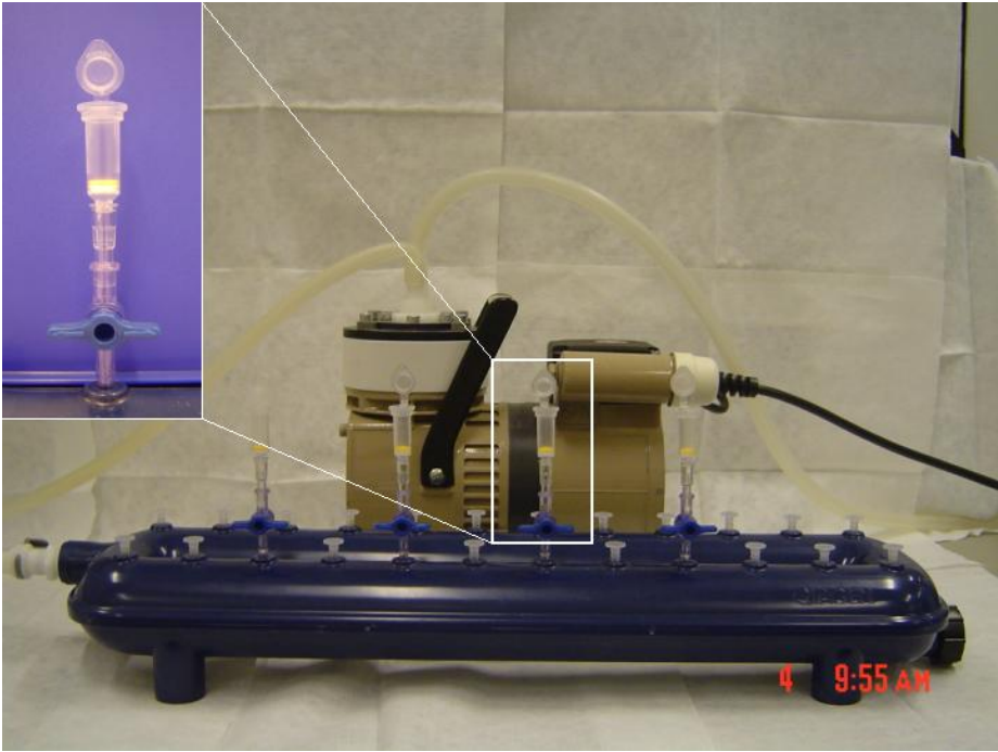
Fig.2-2 The QIAvac 24 Plus, Connecting System, and Vacuum Pump allows collection of fetal DNA and RNA
