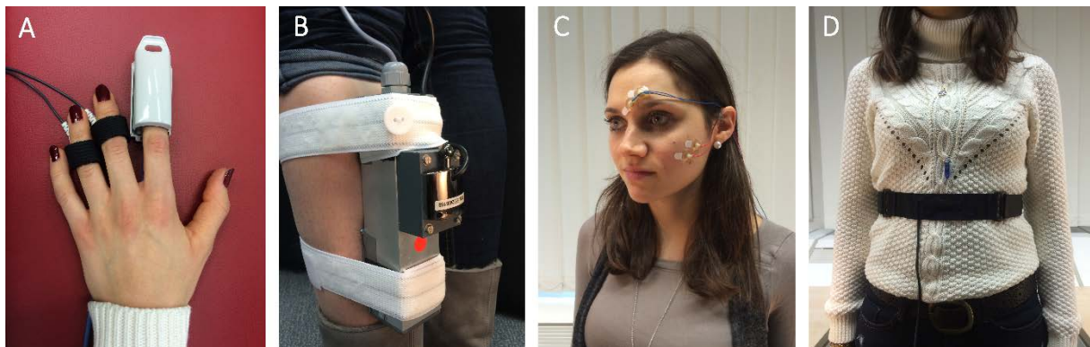
Figure S4. Physiological measures. (A) Measurement of electrodermal activity and blood volume pulse using two electrodes at the phalanges of the ring and middle fingers and a photoplethysmograph sensor on the index finger; (B) collection of piloerection data via a goosecam attached to the lower leg; (C) measurement of electromyographic activity over the corrugator supercilii above the eyebrow and zygomaticus major at the cheek; (D) collection of respiratory activity using a stretch-sensitive respiration belt placed around the diaphragm.
