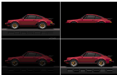
Figure 6.2: Full GIF image (top left), truncated non-interlaced image (top right), truncated interlaced image (bottom left), and reconstruction of this interlaced image (bottom right). Original image from the libungif [53] package, version 4.1.0.
