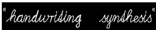
Figure 6.11: Board output generated by handwriting synthesis for the input string "handwriting synthesis".
