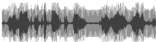
Figure 5.7: Three seconds of a speech signal with a 100 Hz sine-like humming before (light gray) and after filtering (dark gray).
