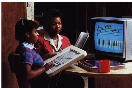
Figure 1.3: The ChalkBoard PowerPad by Chalkboard Inc. was an early example of a digitizer tablet. It was available for the C64 and the Atari 800/XL/XE and came with educational software. Additional edutainment programs were sold for the PowerPad . Each came with a plastic clamshell box to serve as a customized template that was laid over the PowerPad 's surface. Image from [51].
