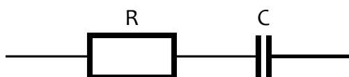
Figure 3.7: RC -circuit as convenient model of the space charge capacitance C_{SC} in series with a linear resistor [26]
