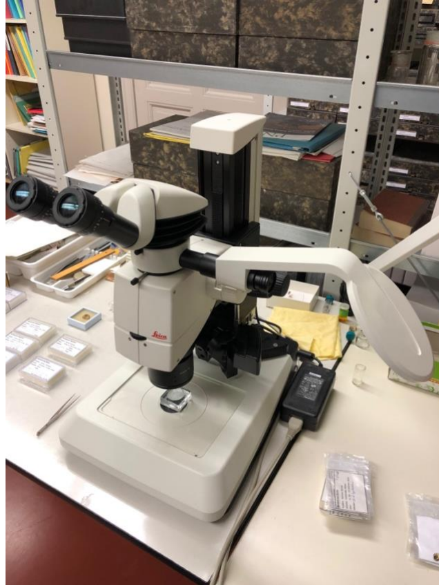
Figure 2.1. Leica M205C stereomicroscope with a camera lucida attachment (photo by Christian Bartel).
